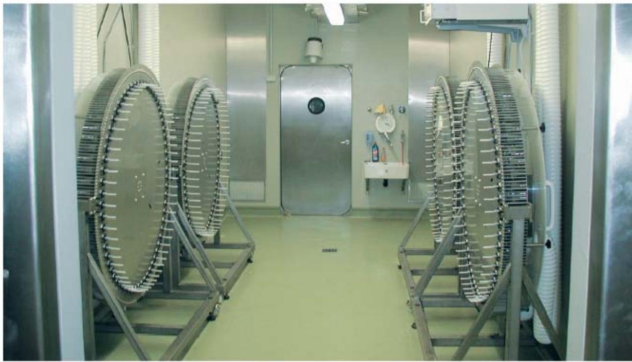
Figure 2 Radio frequency exposure facilities at the Fraunhofer Institute in Germany used in the PERFORM-A project sponsored by Ericsson.
