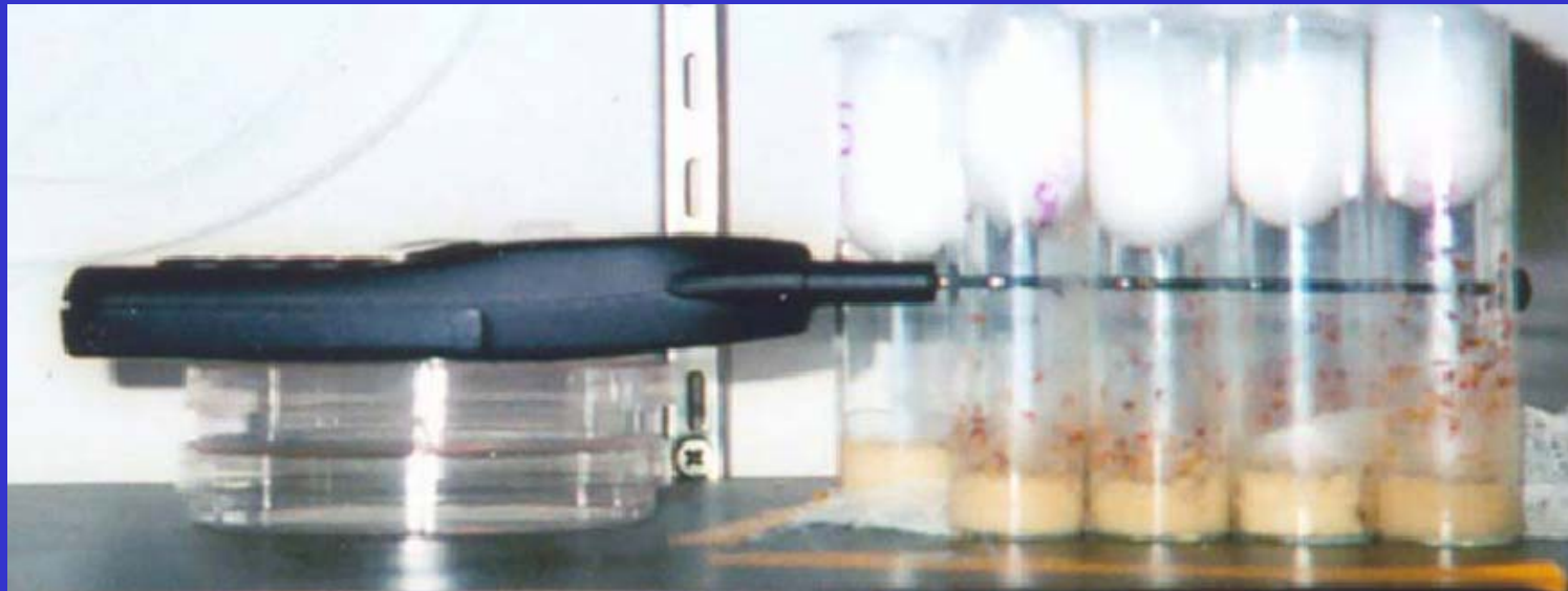
Figure 2 Radio frequency exposure facilities at the Fraunhofer Institute in Germany used in the PERFORM-A project sponsored by Ericsson.
